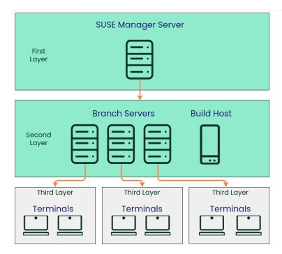
Branch servers should be physically located close to point-of-service terminals, such as in an individual store or branch office. We recommend you have a fast network connection between the branch server and its terminals. Branch servers provide services for PXE boot, and act as an image cache, Salt broker, and proxy for software components (RPM packages). The branch servers can also manage local networking, and provide DHCP and DNS services.
