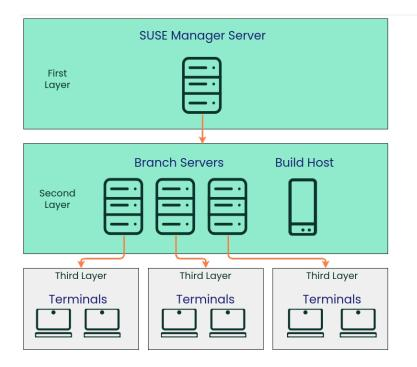
Branch servers should be physically located close to point-of-service terminals, such as in an individual store or branch office. We recommend you have a fast network connection between the branch server and its terminals. Branch servers provide services for PXE boot, and act as an image cache, Salt broker, and proxy for software components (RPM packages). The branch servers can also manage local networking, and provide DHCP and DNS services.
