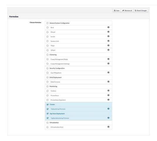
When the formula is activated, navigate to the **Formulas** > **Cluster** tab, and complete the details in the form.
